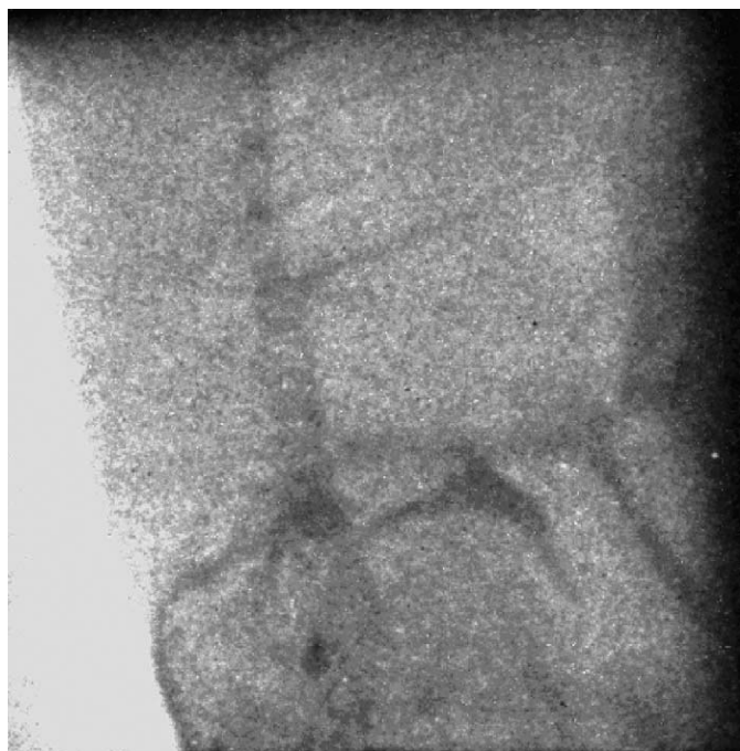
Fig. 9. PXR image of fish bait shown in Fig. 8, 2.6\text{ }\mu\text{A} electron beam current with 15 s exposure.
